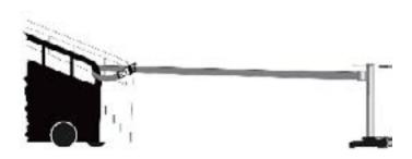
**3.** Loop the belt end through a stationary object and secure the belt end back onto itself to create a temporary barricade.
