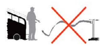
**6. DO NOT** release the belt end with unassisted retraction. **DO NOT** drop the belt end.
